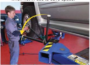
Easily accessible for mechanic to put on or take off tire from the vehicle.
