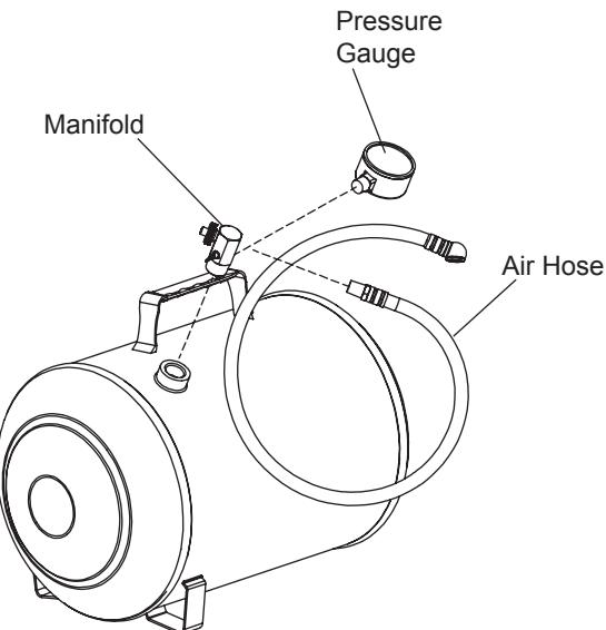
Figure 2 - Air Tank Replacement Parts
